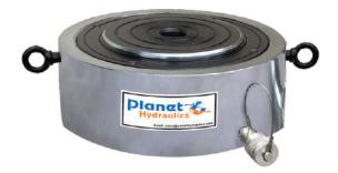
PLPVLS Series - P: Planet, S: Single acting Load return, P: Plain ram, VL: Very Low height S: Spherical saddle (Tilting angle 5° Max), 250 Capacity - ton, 45 Stroke - mm
